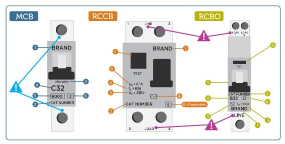
The following must be marked in a durable manner (some may be marked on the side of the device)
