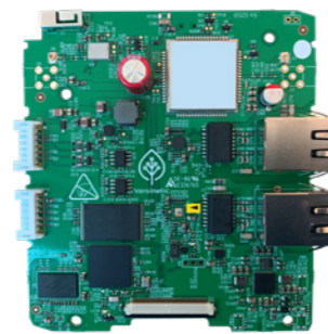
◀ This smart chargepoint communications controller board is an OCPP communications gateway for smart chargers connecting ISO 61851 controllers to back-offices via Ethernet, Wi-Fi or LTE Cellular networks.
