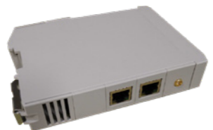
◀ This local controller enables dynamic load management by relaying messages between the charging station's management system and the chargepoint.
