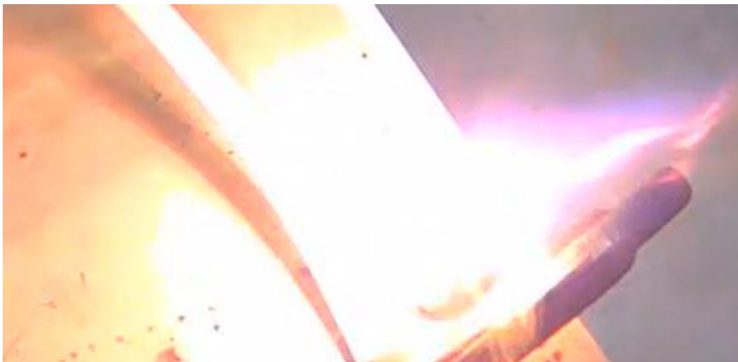
Figure 1-3: ABDX007 (RCBO) XLPE Insulation Cable During Arc Event
