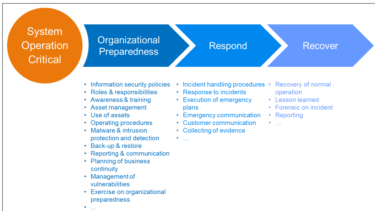
Figure 25: Steps of a Cybersecurity Incident Handling
